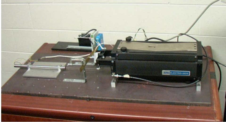
Figure 3: The desktop hybrid platform, used for prototyping and testing Kalman Filter configurations.
