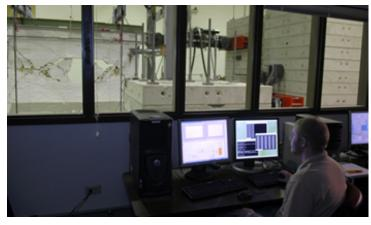
while computer models digitally simulate the physical influence of the structure surrounding the substructure.
