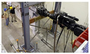
hardware and software, The FHT system consists of three high-speed, high-capacity actuators controlled by MTS 493 control systems, which are linked via a high-speed interface into a real-time computer simulation application. The system features online access to an array of data management and sharing tools, enabling seismic engi¬neers at CU-Boulder to collaborate with peer researchers at remote NEES locations.
