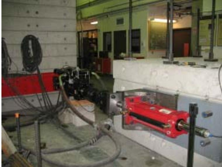
**Figure 18: MR Damper Laboratory Setup**
